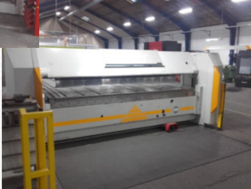
RAS TURBObend Plus (Bending machine) Length: 3200 mm Material thickness: 2,5 mm
