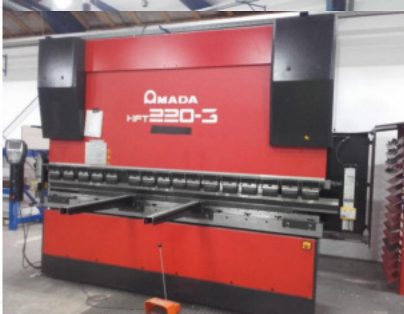
Amada Press brake: Type: HFT 220 tons, length 3200 mm
